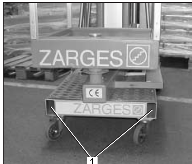
Fig. 44 Installing the outrigger
