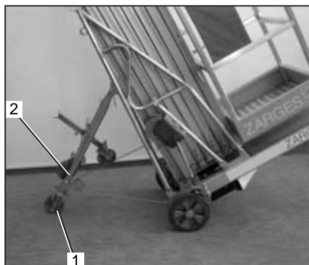
Fig. 46 Tilting the working platform
