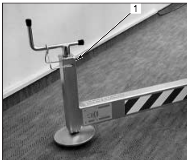
Fig. 53 Grease outrigger spindles
