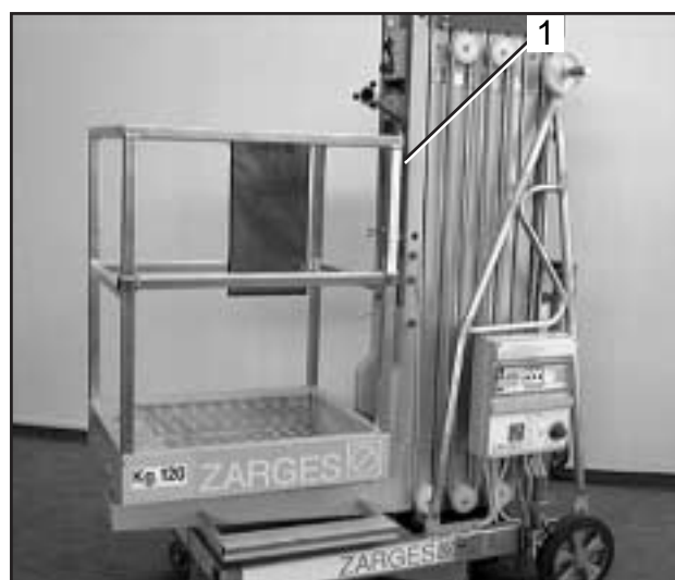
Fig. 40 Removal and installation of rotatable basket
